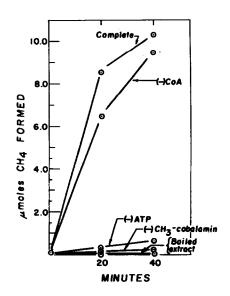
Fig. 1. Effect of ATP on the formation of methane from methylcobalamin. The complete system contained crude extract, 45 mg. protein; potassium phosphate buffer at pH 7.0,500 µmoles; CoA, 0.05 µmole; ATP, 10 µmoles; methylcobalamin, 10 µmoles; total liquid volume 1.3 ml; hydrogen atmosphere; reaction time, 20 min. at 37°C. Values indicate total methane detected per flask.
